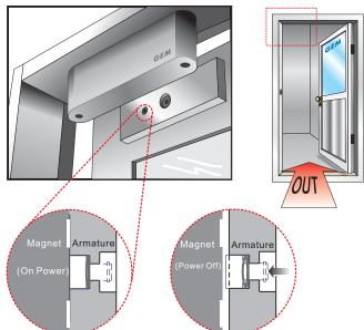
Unique Anti-Residual design When there is no power, there will be no holding force, and the push-off button will pop out immediately, to release the Electromagnetic Lock and the Armature Plate for no residual magnetism.
